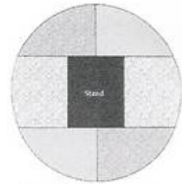
Fig. 6. The cross section of the teapot mould, from the patent specification.
