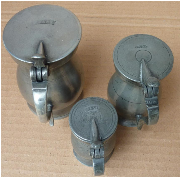
A matching set of three pre-imperial Glasgow Flat-Lid Measures with "GLASS" marl on the lid. Respective capacities 230, 110 & 54ml. The 2 glass is marked by the maker (DS) David Scouler C1819-45 to the upper handle. The number of 1,2,or 4 is not shown, and the 2 spells GLAS with one S. Specialist Collection of Francis Howard (UK PS Member)
