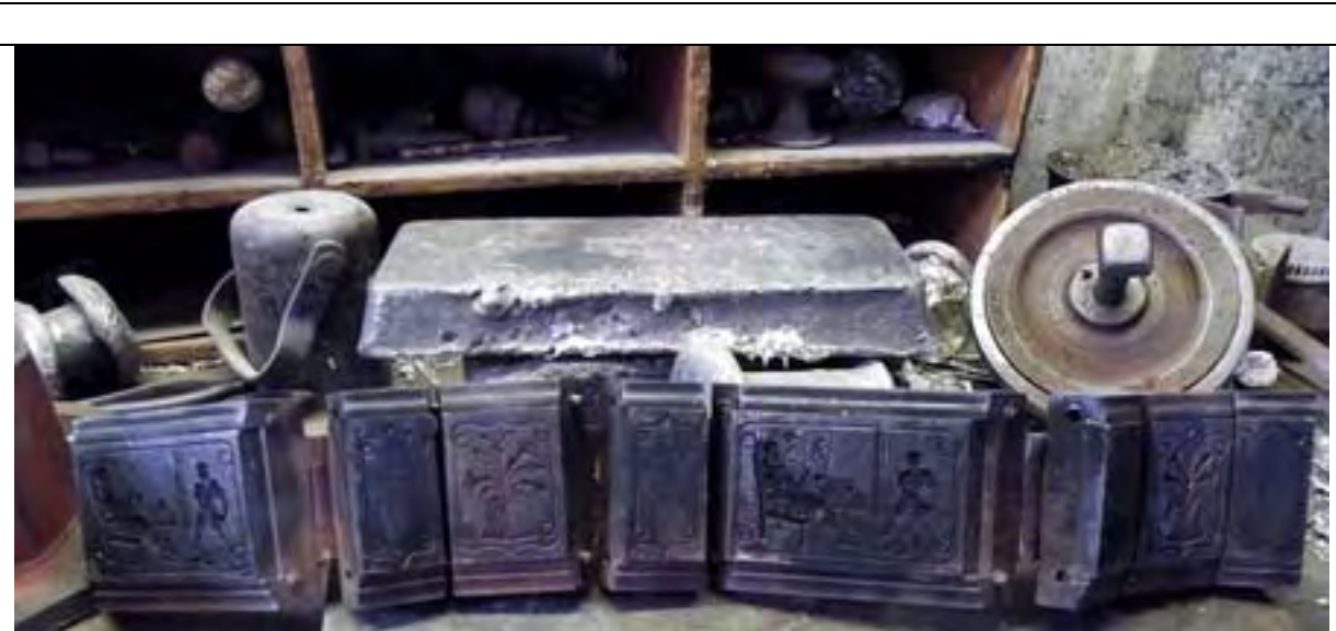
THE RALEIGH TOBACCO BOX – A HINGED MOLD MAKING THE EIGHT SIDES OF THIS OCTAGONAL BOX IN ONE JOINED PIECE – ALTHOUGH SAID ELSEWHERE TO BE 17 TH CENTURY FAR MORE LIKELY TO BE PRE-VICTORIAN SAY EARLY 1800s
