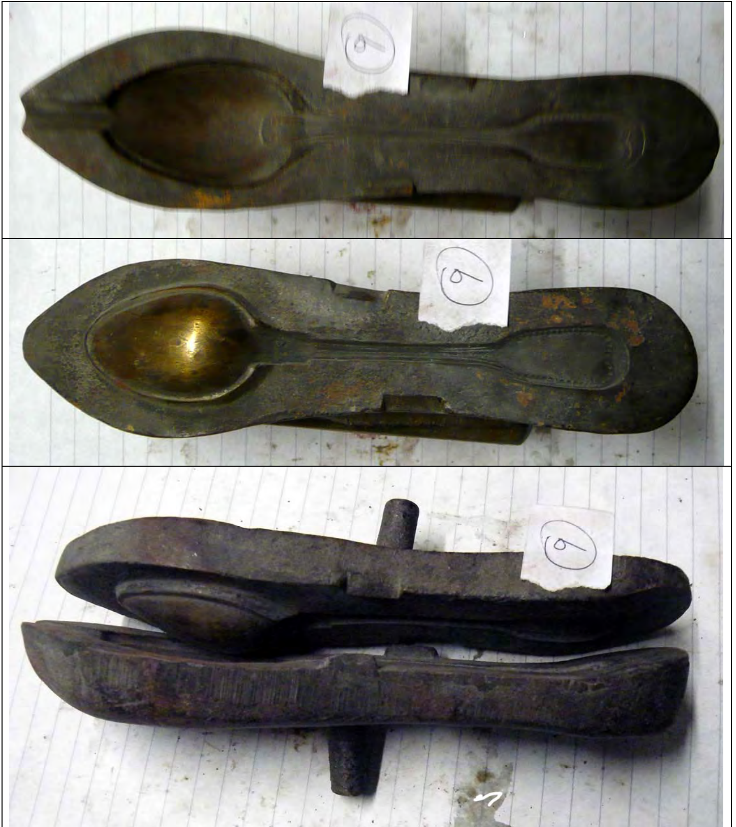
10 – Acorn Knop double mold – modern – length of cast spoon 15.3 cms width 4.5 cms this is a steel mold likely made in the middle 1900s. Q quote from family history “ I’m not casting these one at a time”
