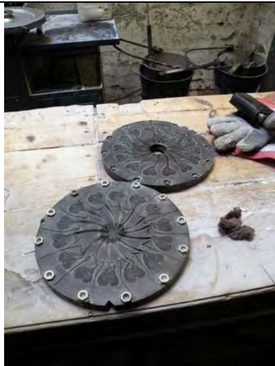
NITRILE MOLDS AS USED IN 2009 – THIS MOLD IS MAKING 20,000 (EVENTUALLY) SMALL TOKENS
