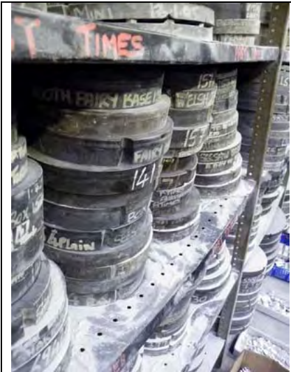
NITRILE MOLDS AS USED IN 2009 – THIS MOLD IS MAKING 20,000 (EVENTUALLY) SMALL TOKENS
