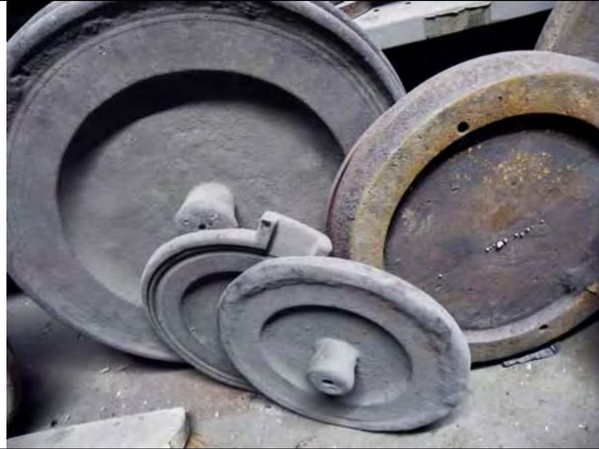
A GALLON HAYSTACK MOLD IN TWO PARTS – THERE WOULD PERHAPS BE A THIRD FOR THE HANDLE. (OR WAS IT A STRAP?)
