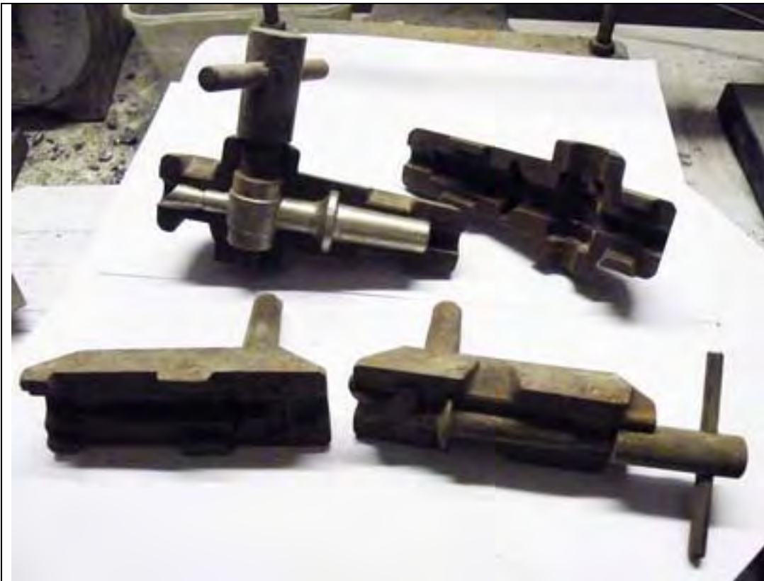
NITRILE MOLDS AS USED IN 2009 – THIS MOLD IS MAKING 20,000 (EVENTUALLY) SMALL TOKENS
