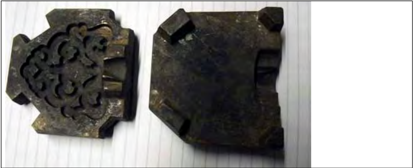
12 – 3 part bronze ½ Candlestick mold for a style known as The Queen Anne Candlestick. The design was popular in that era, the base to this candlestick is oval similar to that of tea pots found then. It is not clear when this mold was made.
